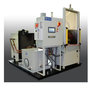
The lower frequency ushered in the leading-edge technology of the Pillar MK-11 power supply. The MK-11 is an IGBT-based power supply with a PLC/HMI operator interface with Ethernet connectivity. The system controls provided all of the part recipe information including the part number being run, tooling part numbers, process parameters and induction coil part numbers. Previously, this information was recorded on set up sheets found on the side of the machine.
