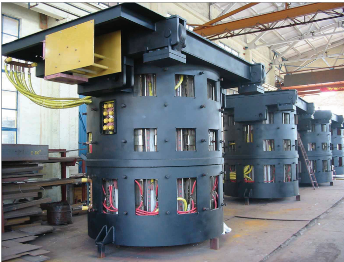
Steel Shell Furnace
