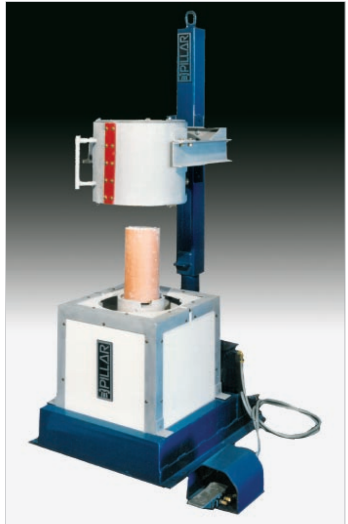
Lift Coil Furnace (Shown in raised position)
